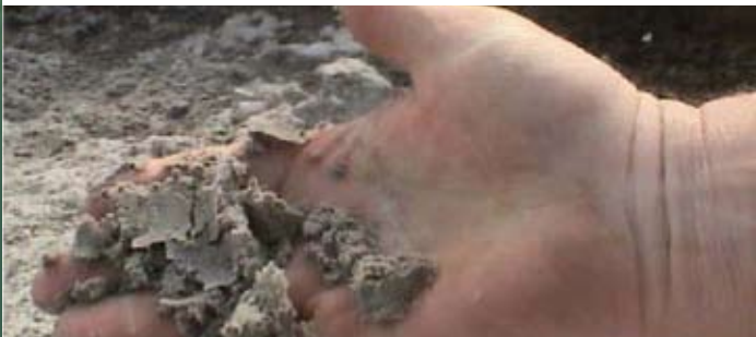
Centrifuge underflow can be set to be as dry or as wet as the operator desires. A wetter underflow will contain less oil on cuttings allowing for easier disposal and greater effectiveness at removal of solids.
