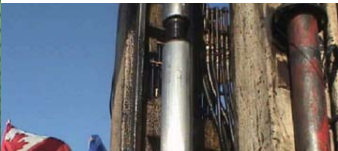
The PolyTar™ system prevents the accretion of bitumen on the drill string.
