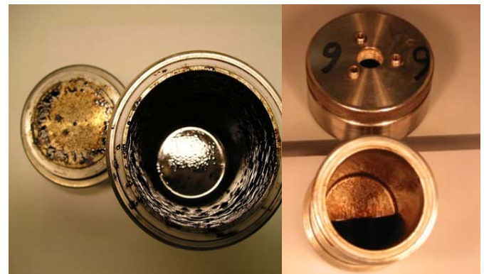
Figure 5 – Accretion forming properties of Fluid without Oil Sands Cleaner (left side) and fluid containing 5% Oil-Sands Cleaner (right side)
