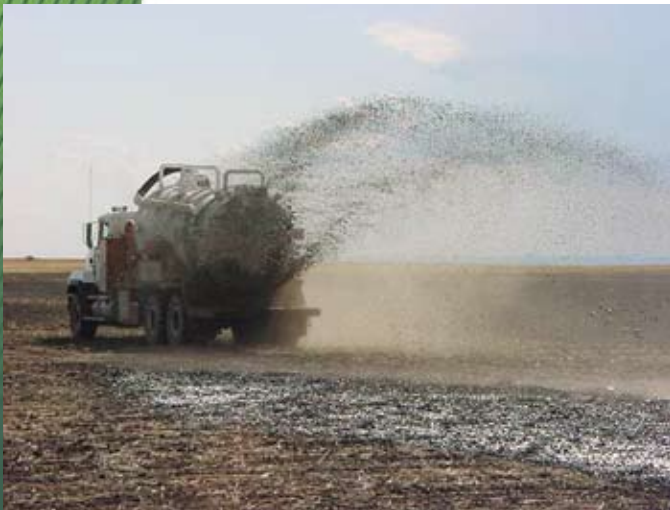
Landspray While Drilling
